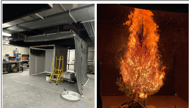
Fig. 5. UMD's Fire hood and example of a burning tree.
