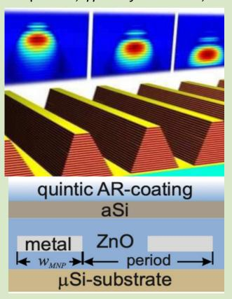
Metamaterial's properties such as light absorption and polarization found to be promising in designing high efficiency solar cells. Antireflection coating of solar cell, made of metamaterial, for example, can block the reflection and increase the efficiency without polarization effect. Nanostructured metamaterials can be also used in the intermediate layers of solar cells with which the band gap can be tuned, thus covering the whole solar spectrum and increasing efficiency.
