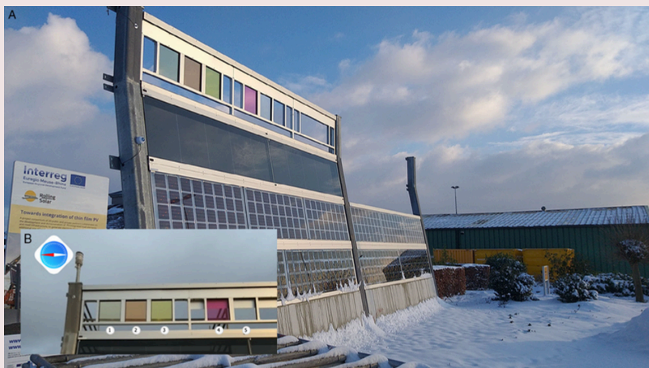
Test setup for outdoor 1-year performance of LSCs based on QDs, https://doi.org/10.1002/solr.202201121
